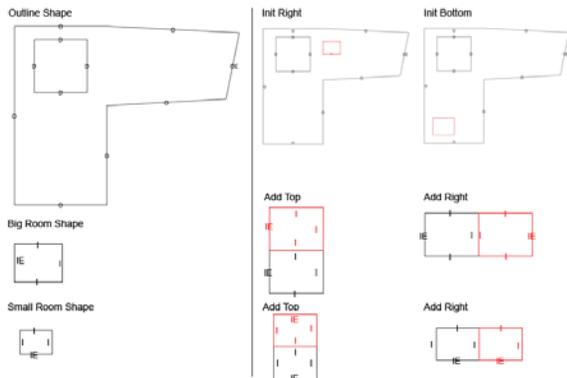
Figure 2: Simple shape grammar for floor plan generation
